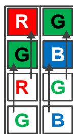
Figure 8-46 Vertical color Binning by 2
