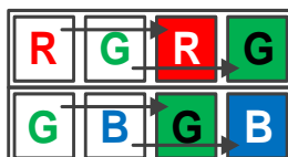
Figure 8-45 Horizontal color Binning by 2
