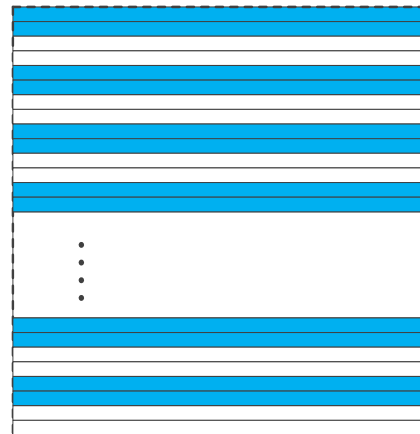
Figure 8-50 Color camera vertical Decimation
